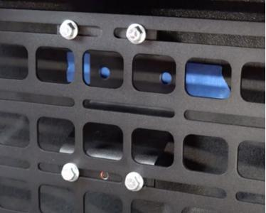
11. To determine where to drill the holes for the front bracket, lift the panel up and make sure the back edge aligns parallel with the tailgate. Do not use the top edge to align as it is not parallel to the bed floor. Once straight, take another piece of painter's tape and place on the bed approximately where you will have the bracket positioned so you can mark where to drill the holes with a pen/pencil.
