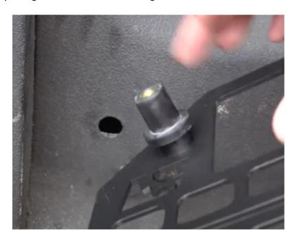
NOTE: If the rubber well nut doesn't seem to fit into the hole in your bed, you may use a sharp knife to bevel the leading edge and insert.
