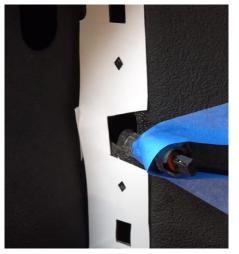
NOTE: If your truck doesn't have the square holes, used the top edge as a reference point. Verify by roughly installing the panel and seeing that the lower mount and your marked drill poins align with the panel.
