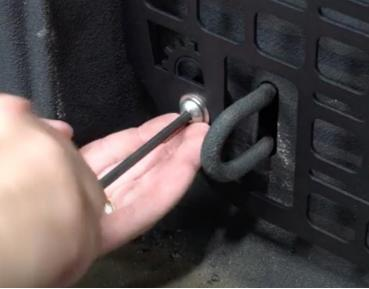
15. Next, we'll tighten the rubber well nut in the lower rear position of the panel. This doesn't need to be too tight, just snug to keep the panel from swinging out away from the bedside (above).
